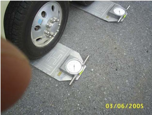
Knowing the total weight of our coach is interesting and important. Knowing the load carried at each wheel station tells us if we have stowed the coach incorrectly and have one or two wheels carrying too much weight or tires under are inflated for the weight on the wheels.
