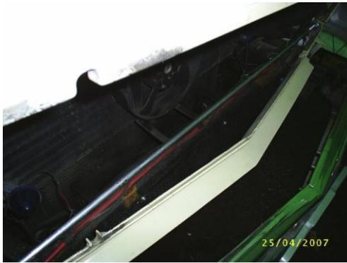
A bonus was being able to centre the coach frame and the fenders by turning the nuts varying amounts on each.
