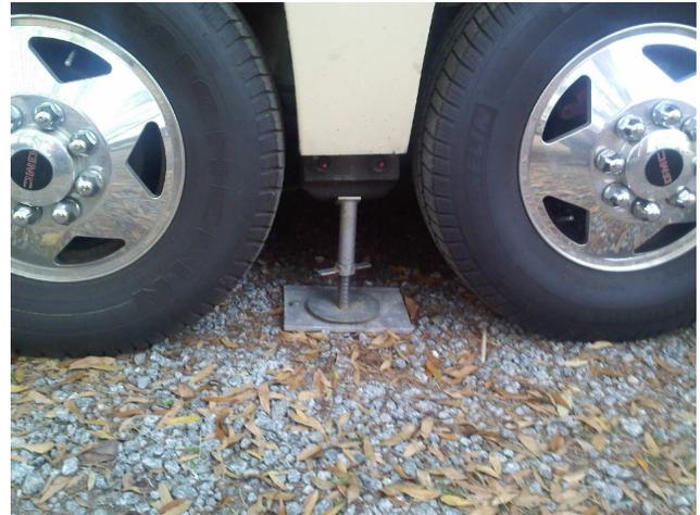
If you are having a problem with the air suspension system leaking down in cooler weather or when parked for two or three weeks, these small, yet adjustable stands work very well. The circular base needed to be replaced with a heavier plate to hold the weight of the coach. They are sold in Vendors Row at the GMC Motorhomes International Conventions.
